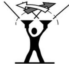
LZ UNSAFE (NIGHT)
