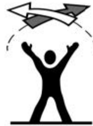
LZ UNSAFE (DAY)
